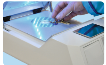
2. Put sample on the analytical window
